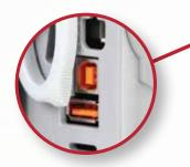
USB ports for printer, RFID reader and web camera support
